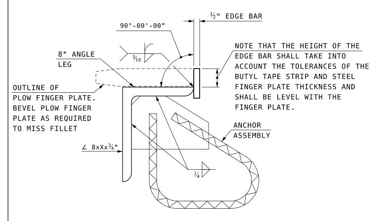
PLOW PROTECTION PLATE EDGE BAR DETAIL (ANGLE)
